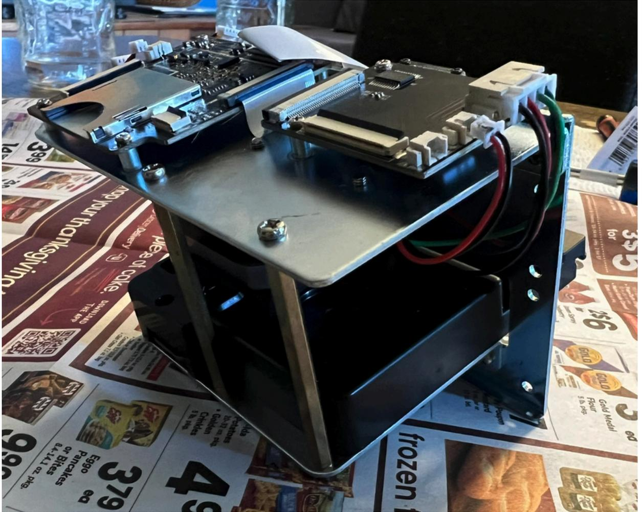
11. We'll be focusing on the board with the SD card slot. First remove the two ribbon cables connected to this board, there is a cable going to the camera and a cable going to the side board.
