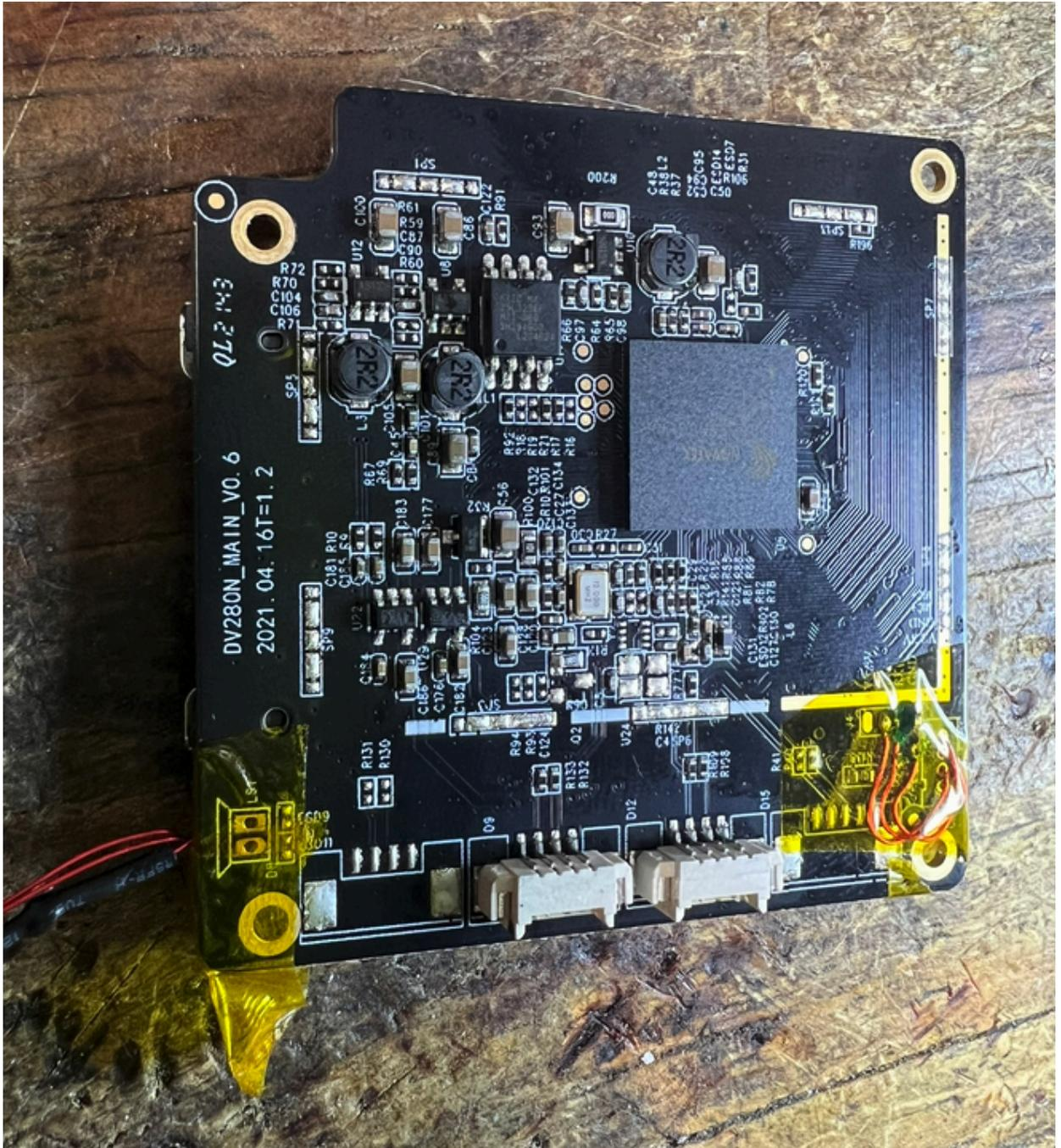
16. Connect the three wires to your UART to the USB serial adapter or an Arduino nano board. See the documentation that came with your adapter for specific details.
