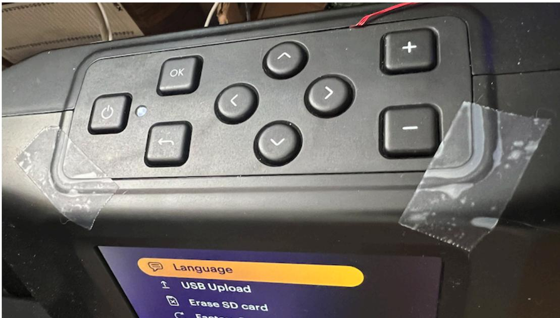
3. Carefully pry apart the two halves of the case - **DO NOT FULLY separate the case yet.** You should not need to use a lot of force, but some of the plastic edges can get stuck. If you run into trouble, ensure all 8 screws are removed.
