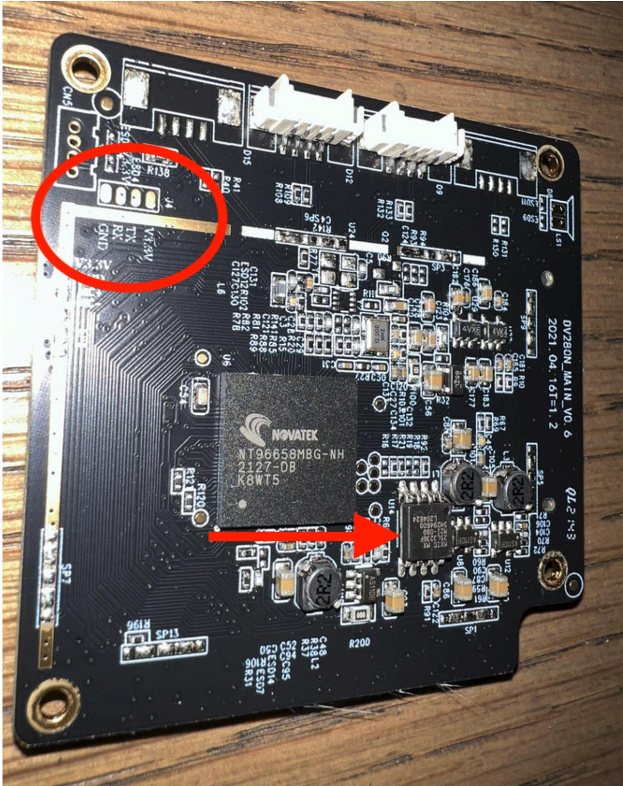
14. You'll only need to solder three wires to GND, RX, and TX. You **do not** need to solder a wire to **V3.3**. I used 34 AWG sized enameled wire for this task, but any thin wire will do.
