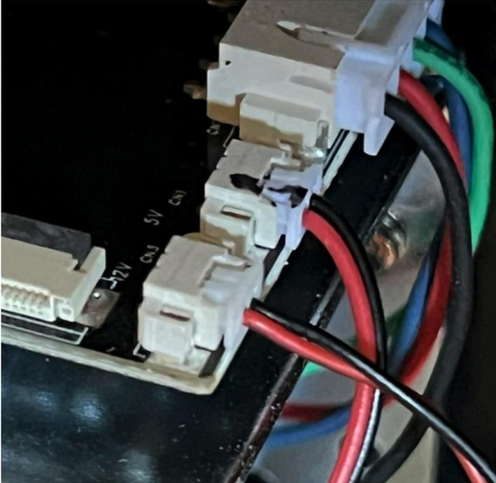
7. Carefully remove all of the non-ribbon cables plugged into the left side of the board. Most of the cables on the right can stay in place except for one black and red pair.
