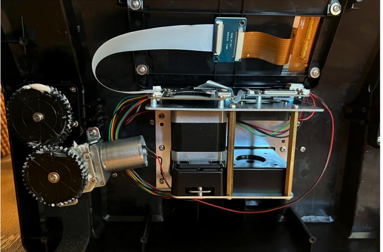
6. The scanner has a lot of similarly colored wires. You may want to mark these with a marker by putting a smidge of color onto the connector where it meets the cable. This way you can determine which plug goes where.
