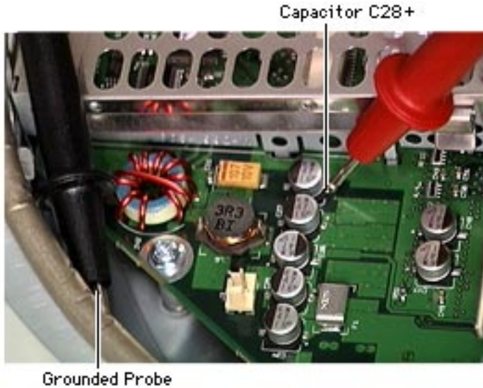
Testing for Power at the Logic Board
