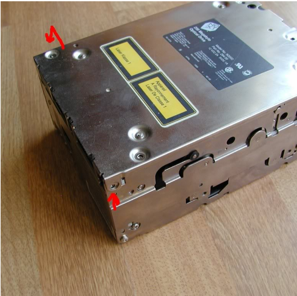
Remove these two screws that act as hinges for the PCB assembly.
