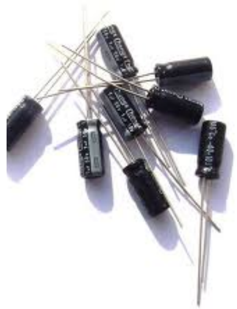
Approximately 29 aged Electrolytic capacitors must be replaced, depending on Motor Board revision.
