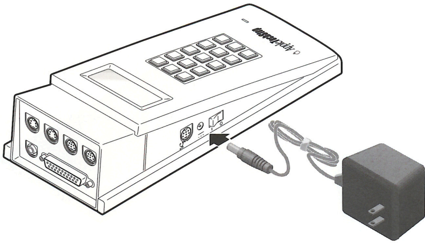
Figure 3-5 Attaching the AC Adapter
