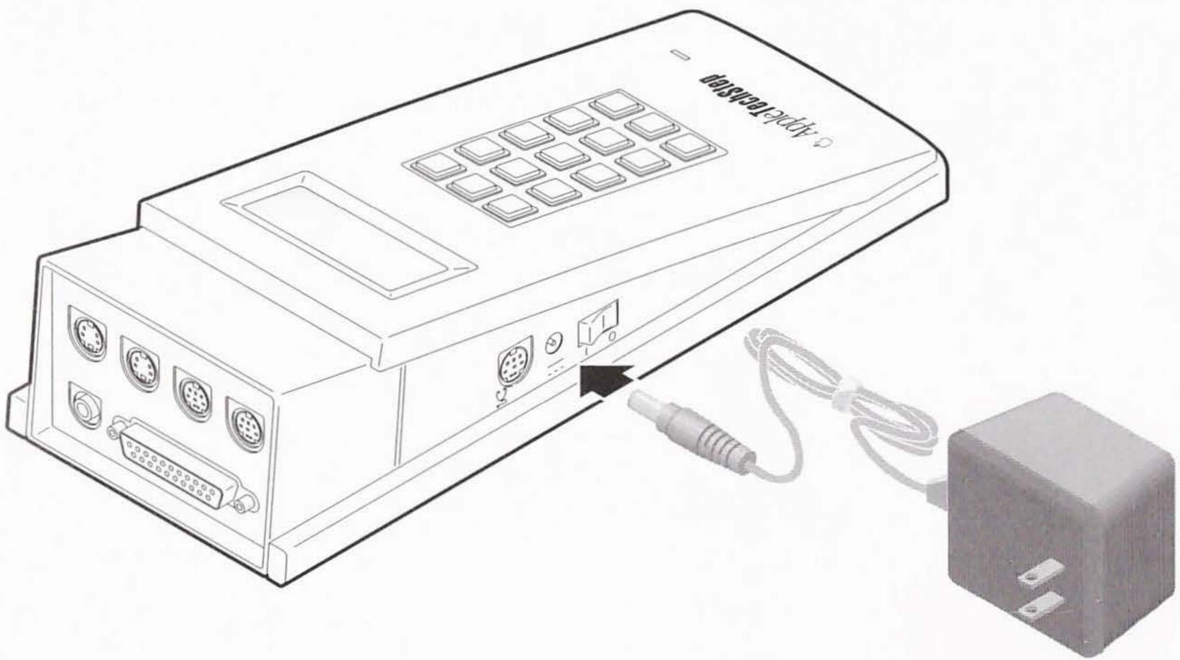
Figure 3-5 **Attaching the AC Adapter**
