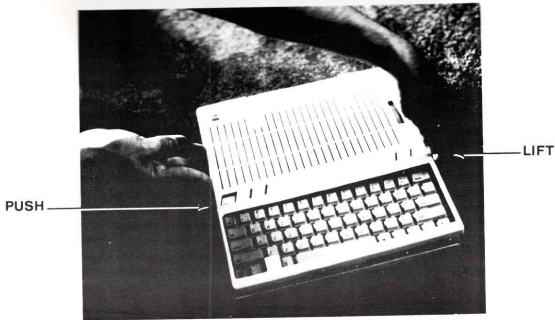
Push on the top cover (the side with the Apple logo) and lift on the other side (the disk drive side). At the same time, loosen the back panel which is a separate piece. On some IIC's this may require a bit of wiggling, but it will come off. If you break any snaps, don't worry as there are twice as many as necessary.
