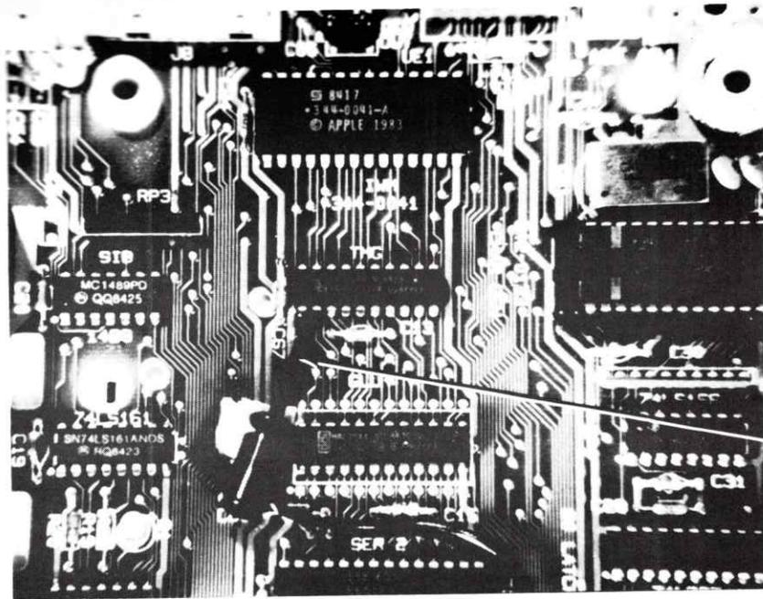
There is a short wire connected to the Z-80c card. On the end of this wire is a small plastic "grabber". When you press the grabber together, a metal hook will project out of the housing. Hook the grabber to pin 2 on the "TMG" I.C. Use the small piece of double sticky tape provided to hold the grabber down flat.
