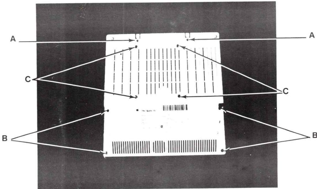
Turn the IIc upside down and using the Phillips screwdriver, remove the screws indicated as A, B and C. The A, B and C screws are of different thread types so keep them separated so that you can reinstall them in their original positions as shown. Some of the screws may not unscrew completely, this is normal.
