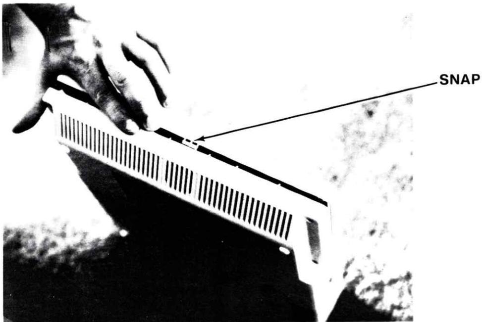
Should the snap break off, it is of little consequence as it is only used by Apple so that they can put the IIC together a few seconds faster. When you reassemble the IIC, the screws on the back hold it together firmly.
