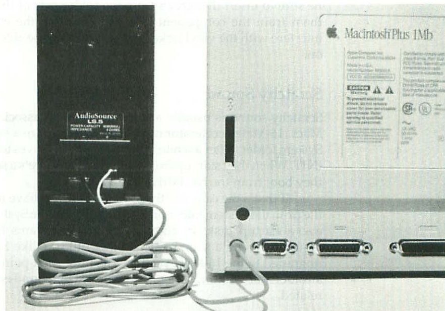
Figure 8-3 External speaker connections for the Macintosh Plus.
