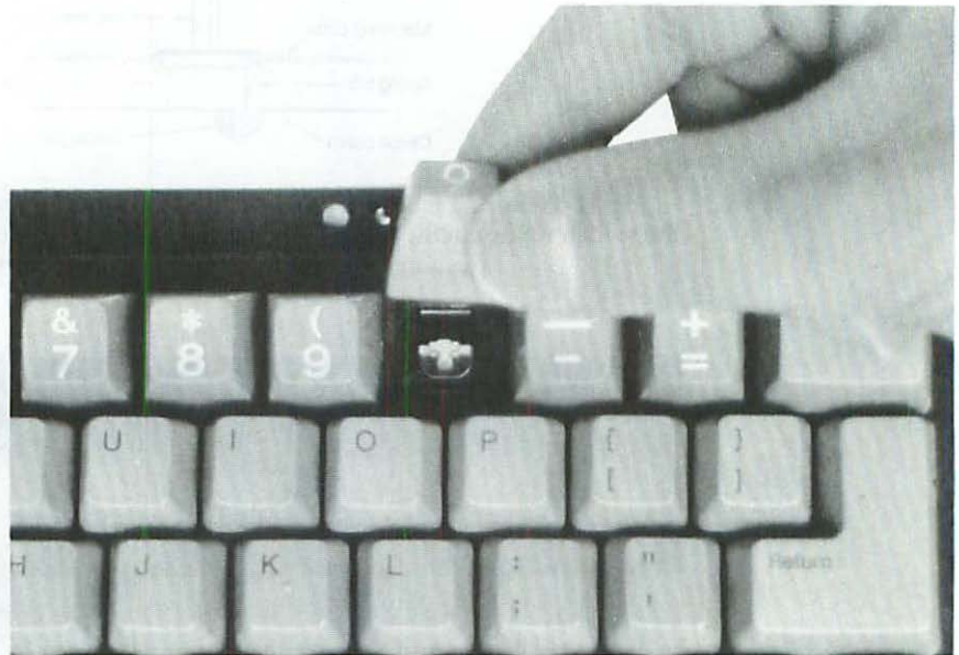
Figure 11-14 Replace the cap, resolder the tails and you're all done!
