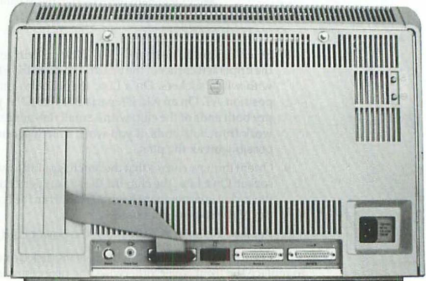
Figure 13-28 On the Lisa 2/5, internal hard drive upgrades plug into an external connector.
