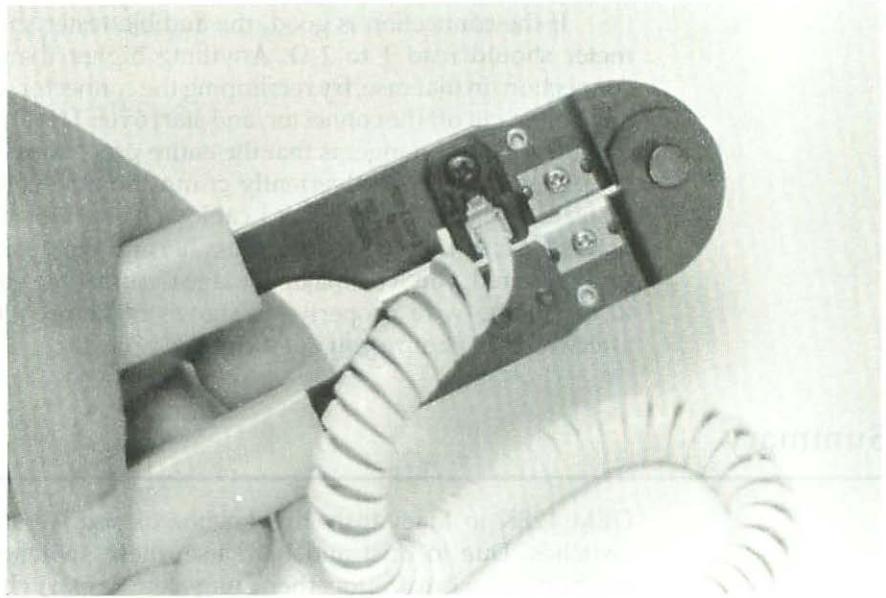
Figure 11-20 Crimping a new connector.
