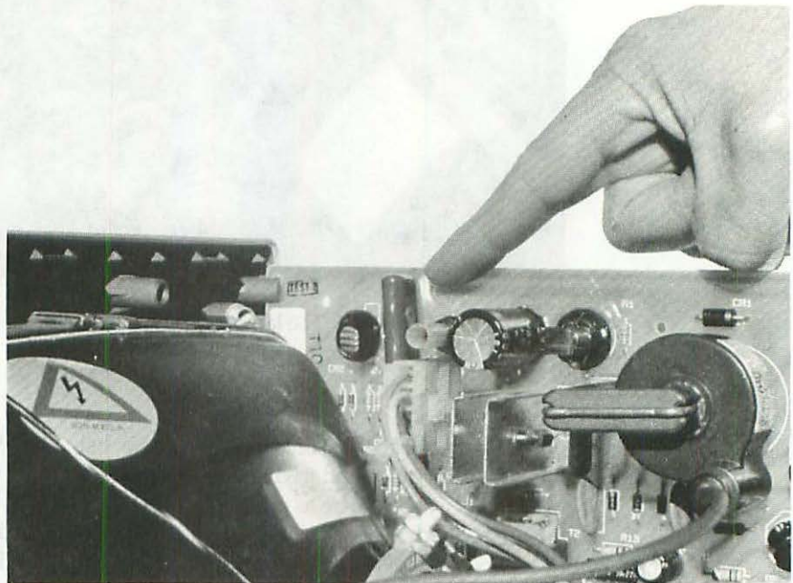
Figure 5-8 3.9-mfd 100-V metallized-polyester caps can also be used.
