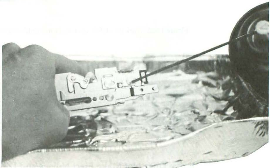
Figure 13-21 Spray away the old grease with WD-40.
