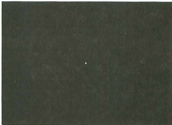
Figure 5-22 No horizontal sweep. No vertical sweep. This display suggests that the CRT to J1 cable is disconnected.
