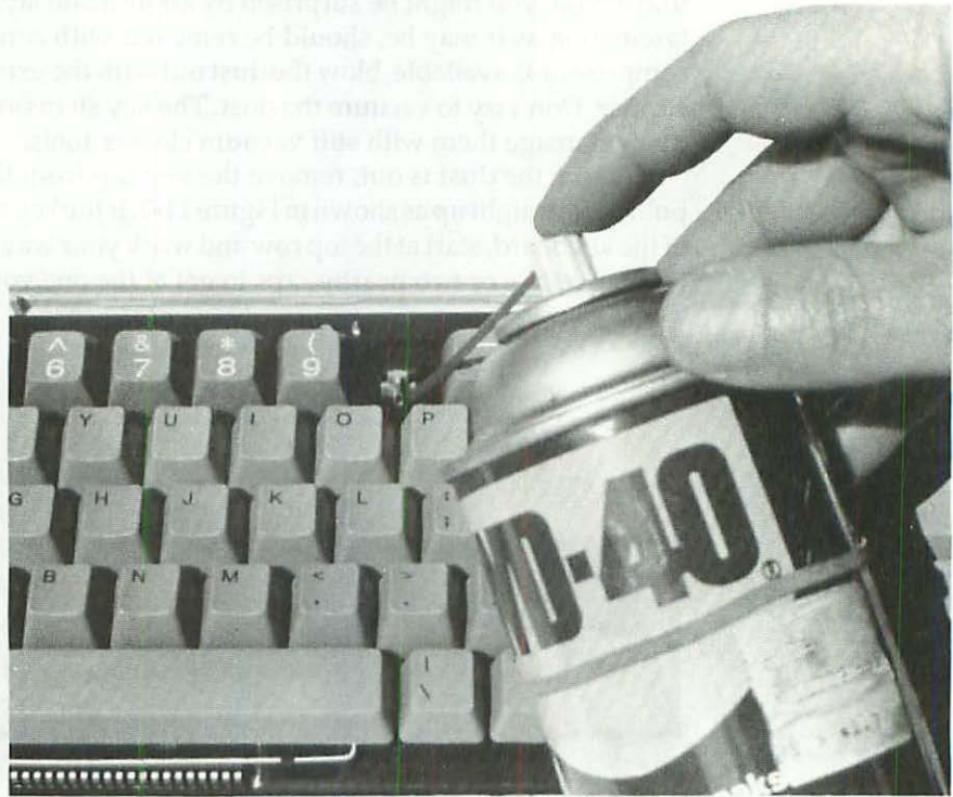
Figure 11-3 Intermittents can be treated with WD-40.
