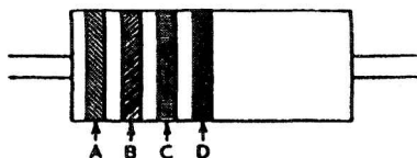
Figure 24.1 Ring colour code for resistors
